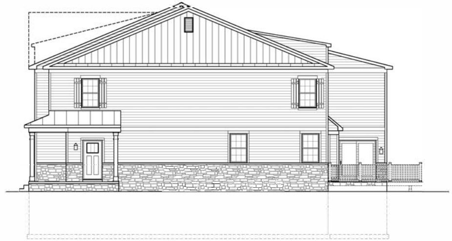
RIGHT SIDE ELEVATION (HI-VIZ) IN-GROUND BASEMENT- WATERTABLE
